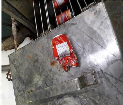
Gambar 2.13 Cacat *knocked down flange*
