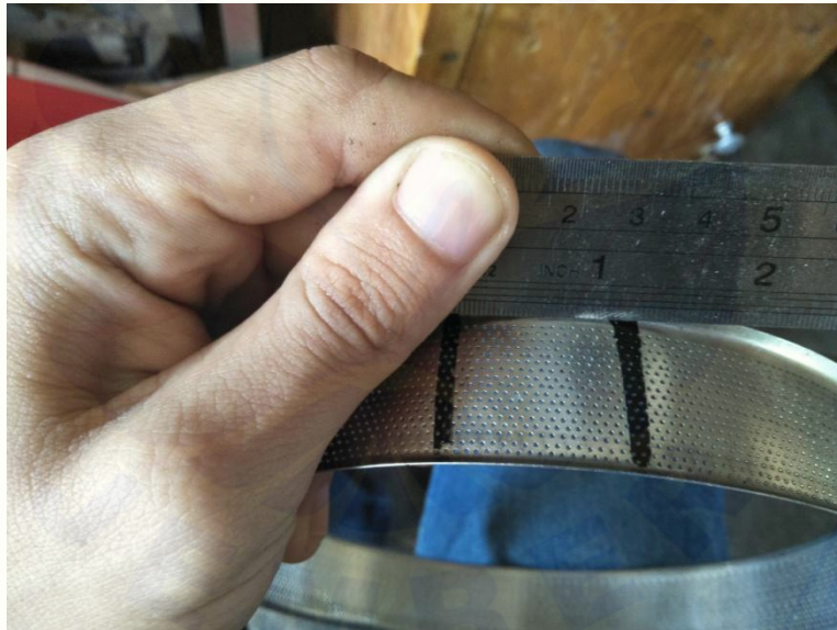
Gambar E.3 Saringan Disc Mill ukuran 1 inch 2 = 98 lubang, diameter lubang 0,3 mm
