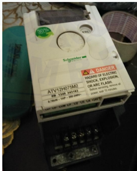
Gambar E.5 Variable Speed Drive
