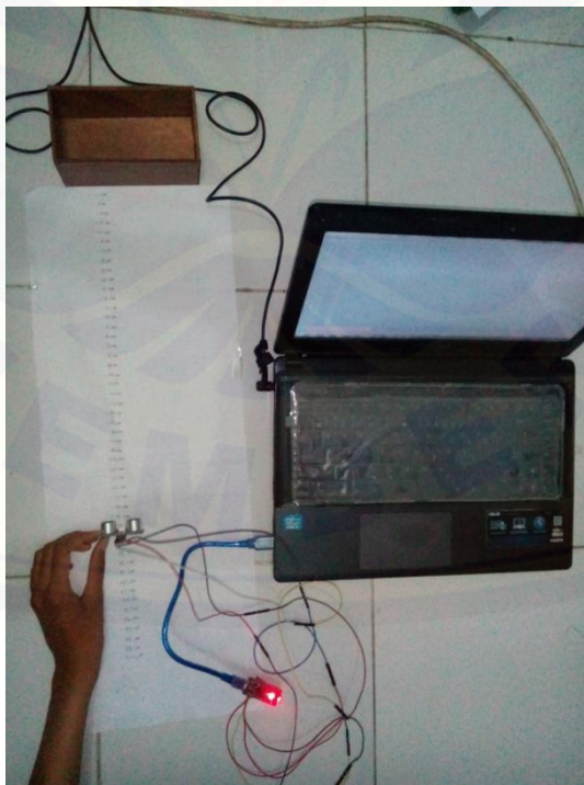
Gambar A.2 Kalibrasi Sensor Ultrasonik HC-SR04
