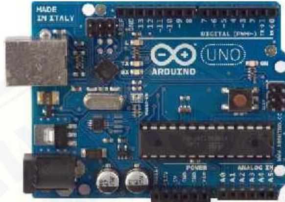
Gambar 2.3 Board Arduino UNO (Sumber : Azzi Taufik, 2014)
