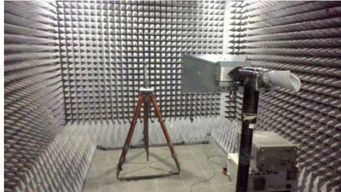
Gambar 6. Proses Pengujian di Ruang Anechoic Chamber
