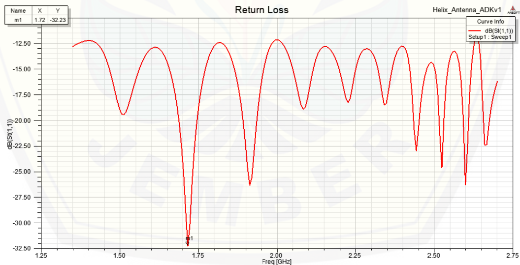
Gambar 3.11 Grafik Return Loss Antena Helix Mode Axial
