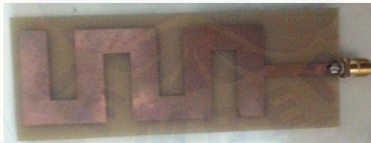
Gambar 3. Antena Patch Meanderline DGS Tampak Atas
