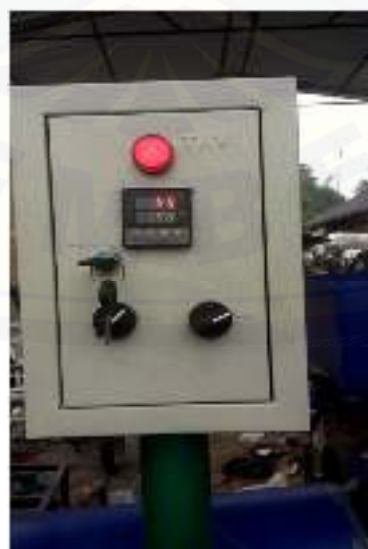
Gambar C.19 Temperatur pengeringan mesin rotary dryer
