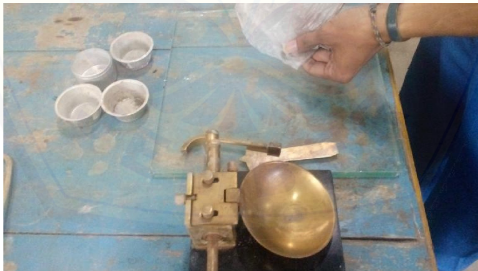
Lampiran 1.6 Gambar Pengujian Atterberg Limit
