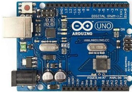
Gambar 3. 5 Arduino Uno R3(Sumber Arduino.cc)
