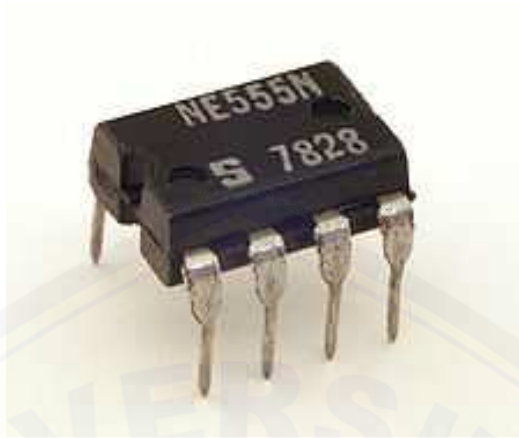
Gambar 2.3 IC NE555 ( https://en.wikipedia.org/wiki/555_timer_IC )
