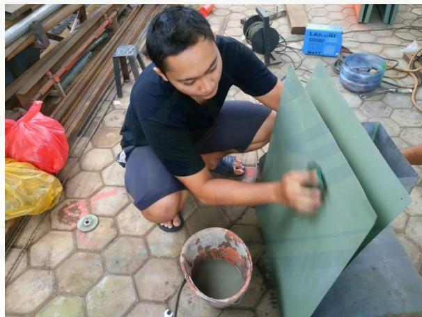
Gambar C.41 Proses Penghalusan Cat Dasar
