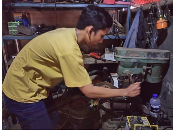
Gambar C.15 Proses Pengeboran Dudukan Reducer
