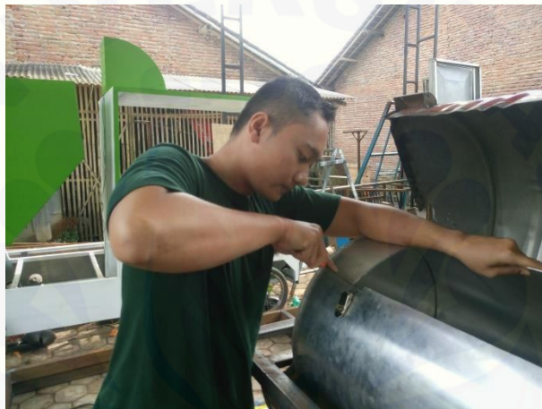
Gambar C.28 Proses Pengikiran Pinggiran Tabung
