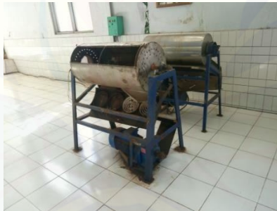
Gambar 2.9 Rotary Dryer di PTPN XII Kebun Kertowono
