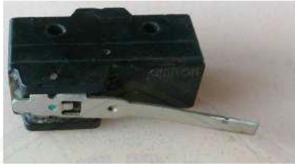
Gambar 3.3 Limit switch tipe Z-15GW-B.
