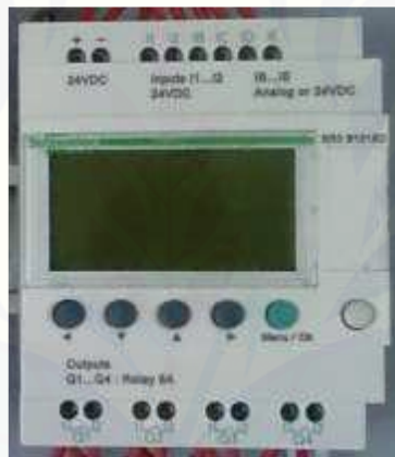
Gambar 3.2 PLC Schneider tipe SR3B101BD.
