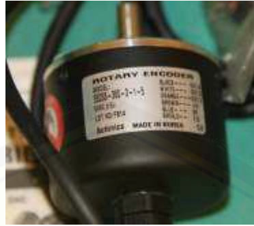
Gambar 3.5 Rotary Encoder E50S8-1000-3-T-24 Autonics.
