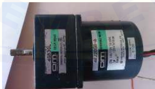
Gambar 3.11 Motor listrik 4RJ20GB-A Oriental Motor.
