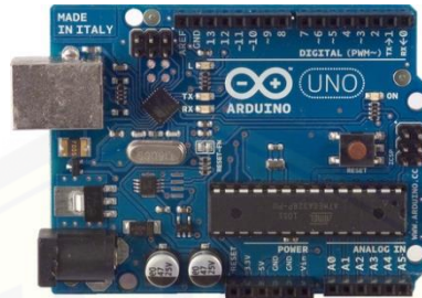
Gambar 2.2 Board Arduino Uno (Sumber : Taufik, 2014)
