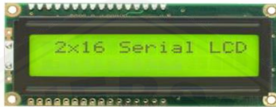
Gambar 2.12 LCD ( Liquid Crystal Display ) (Sumber : Arini, 2015)
