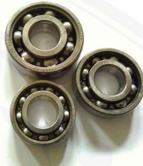
Gambar 3.8 Bantalan uji ( Single Row Deep Groove )
