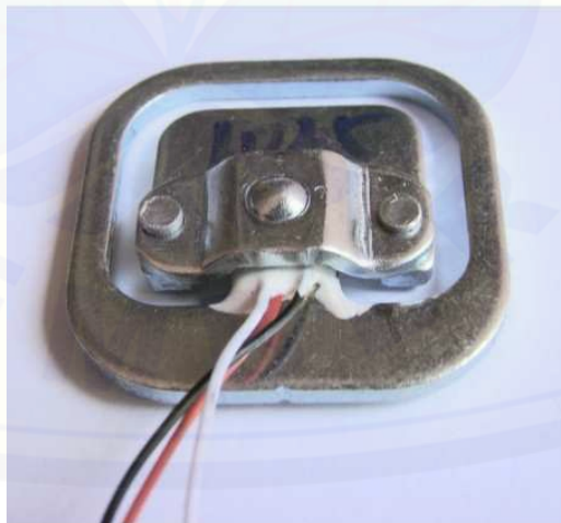
Gambar 3.3 Load cell 50 kg
