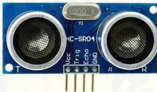
Gambar 2.4 Sensor Ultrasonik HC-SR04 (sumber : Santoso, 2015)
