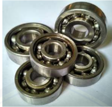
Gambar 3.8 Deep groove ball bearing (Sumber: arsip pribadi)
