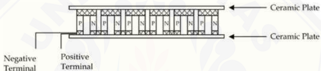
Gambar 2.9 Modul thermoelectric (Sumber: Gould dan Shammass, 2009)
