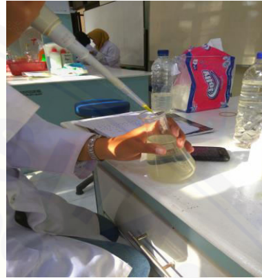
Gambar 14 Penetesan Indikator K_2CrO_4 5%
