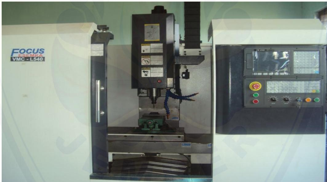
Gambar 3.1 Mesin CNC *Milling* FOCUS ESEMKA VMC – L540
