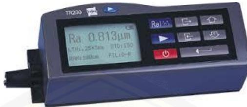
Gambar 3.5 *Surface Roughness Tester*
