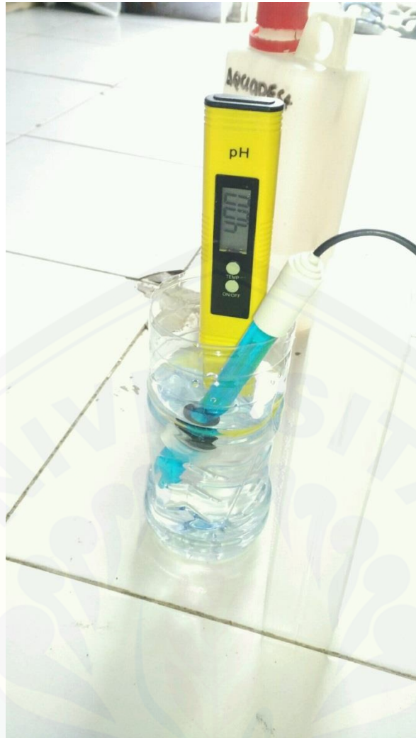
Gambar 6 Proses kalibrasi sensor PH DF Robot v 1.1
