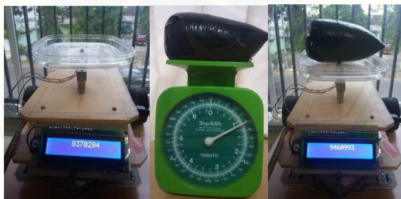
Proses Kalibrasi Load Cell
