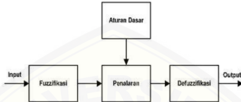
Gambar 2.2 Blok Diagram Logika Fuzzy (Sumber : Nugraha (dalam Mahagiyak dkk, 2013) )
