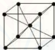
Gambar 2.3 Struktur kristal body centered cubic (Sumber: Kittel, 1996)
