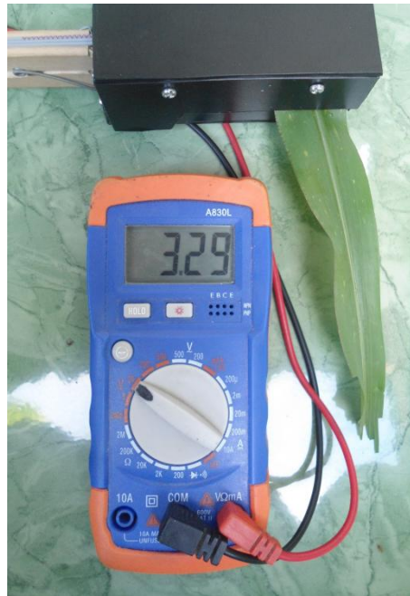
Gambar 4.8 Tegangan Photodioda Saat Terhalang Daun Tanaman Jagung
