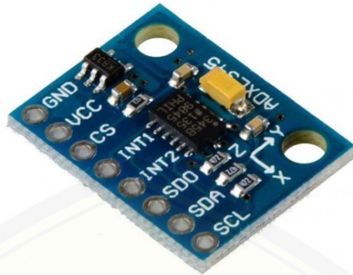
Gambar 2.6 Rangkaian sensor ADXL345 ( http://id.aliexpress.com/ )
