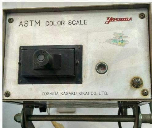
Gambar 9 ASTM Color Scale
