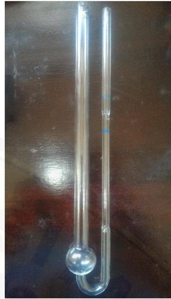
Gambar 8 Viskometer
