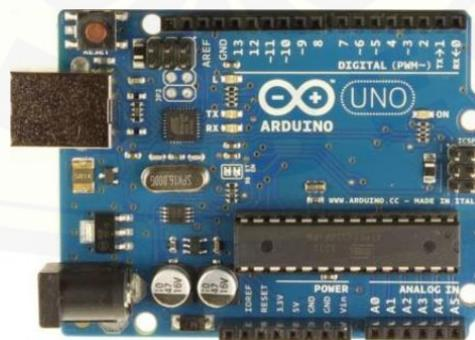
Gambar 2.8 Board Arduino Uno (Sumber: Anwar, 2015).
