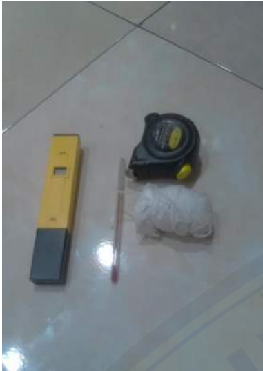
Gambar 1. Peralatan (Phmeter, termometer, meteran gulung, benang)
