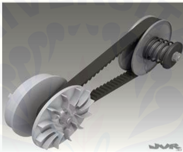
Gambar 2.4 CVT Matic (Sumber JVR Racing.Com)
