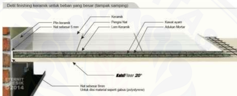
Gambar 2.5 Detail Finishing Tampak Samping
