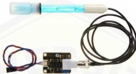
Gambar 2.4 Analog pH meter kit (Robot Wiki, 2014).
