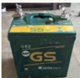
Gambar 2.14 Baterai lead acid 12V
