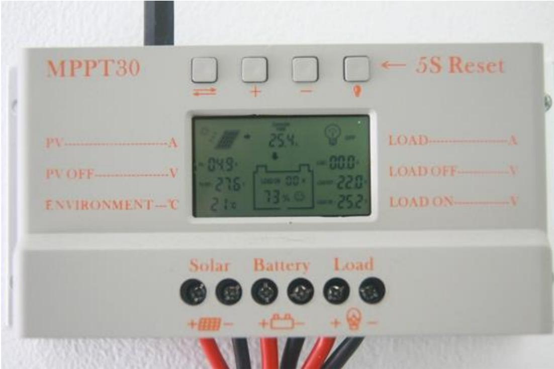
Gambar 2.2. Solar Charge Controller MPPT 12/24 volt (Auto), 30 A.
