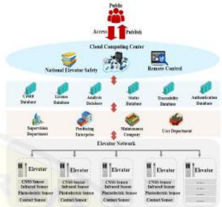
Fig. 2. Elevator Network Security Monitoring Service Platform
