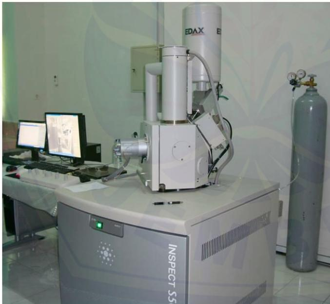
Alat *Scanning Electron Microscope* (SEM)
