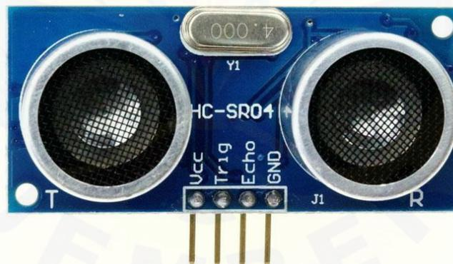
Gambar 2.2 Sensor Ultrasonic HC-SR04
