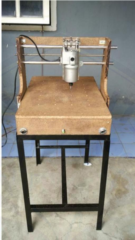
Gambar C.9 Mesin CNC Router Milling tampak depan
