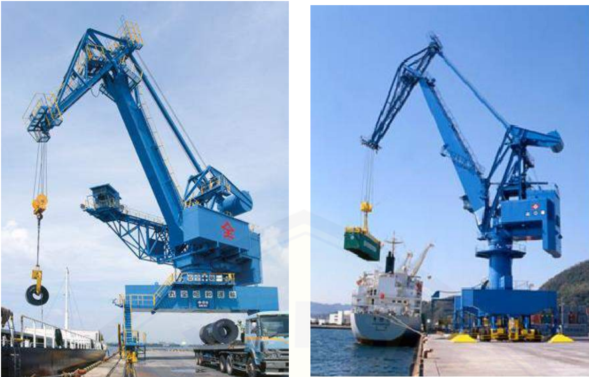
Gambar : Gantry Luffing Crane (GLC)
