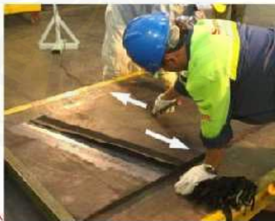
Gambar 3.14 Proses stitching (Sumber: Summa Learning Center )
