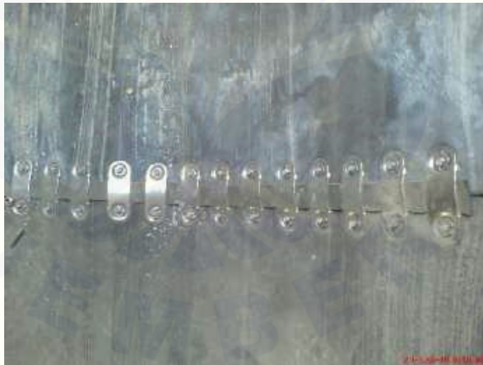
Gambar 2.11 Penyambungan Mechanical System (Sumber: Summa Learning Center)
