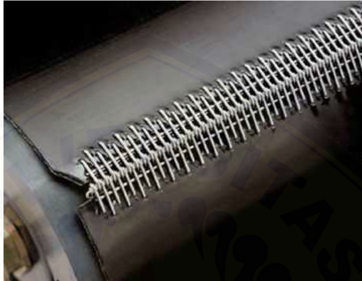
Gambar 2.10 Penyambungan Fastener Belt Conveyor (Sumber: Flexco)
