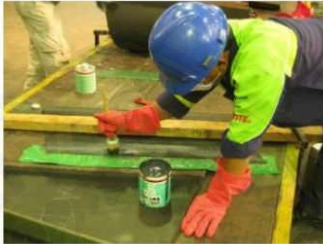
Gambar 3.13 Pelapisan lem (Sumber: Summa Learning Center )
