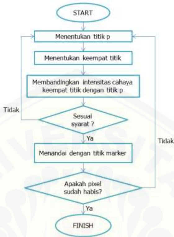
Gambar 2-6 Diagram alir algoritma FAST Corner Detection
