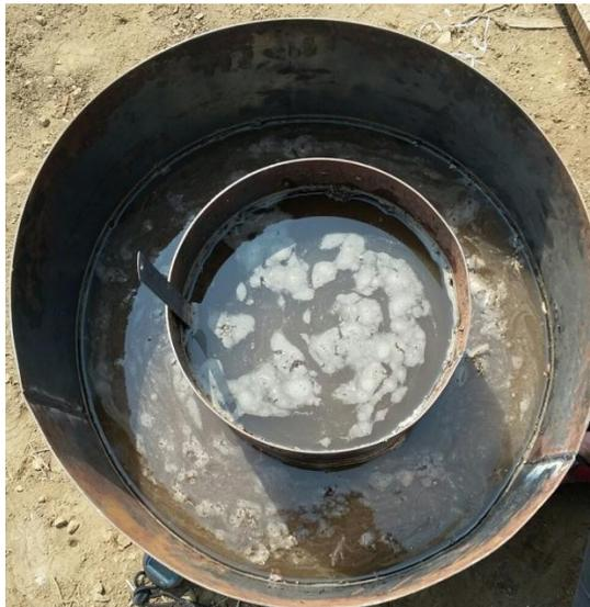
Gambar 3.2 Alat Double Ring Infiltrometer
