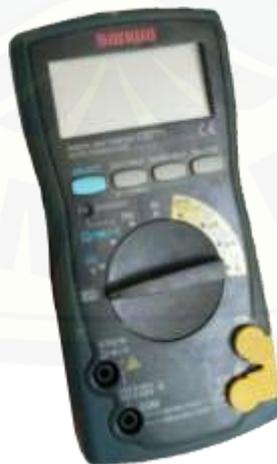
Gambar 3.4 Digital Voltmeter Sanwa CD771
