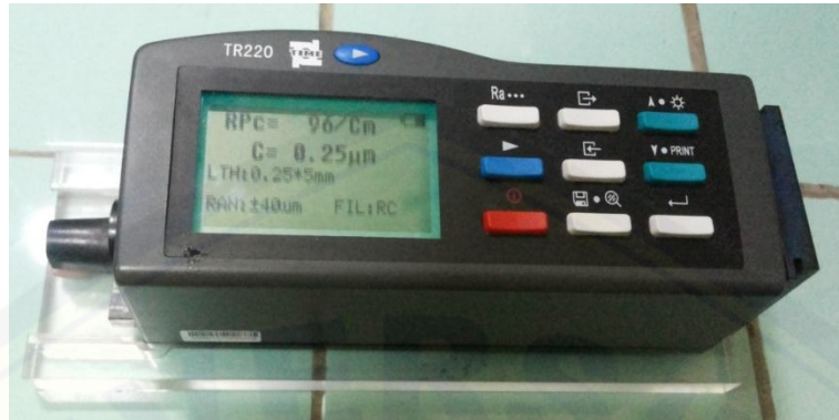
Gambar 3.8. Surface Roughness Tester (TR 220, China) (Sumber: kusumawati, 2012)
