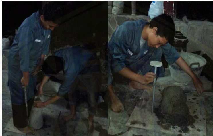
Gambar 4.2 Proses Pengujian Slump
