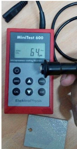
Thickness gauge test
