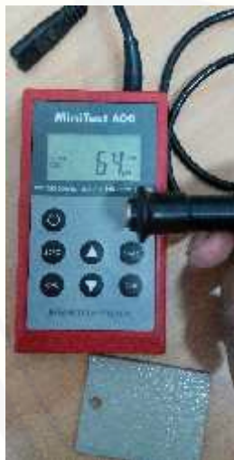
Thickness gauge test
