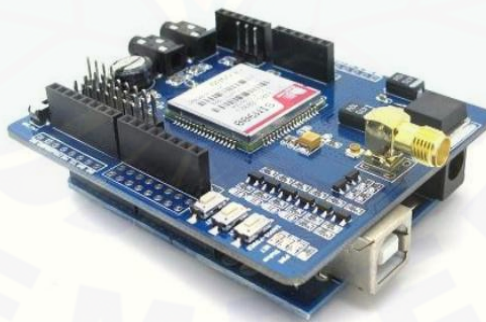
Gambar 2.11 IComSat v1.1 SIM900 GSM/GPRS shield
