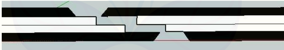
Gambar 3.14 Pencocokan ujung belt (Sumber: Summa Learning Center )
