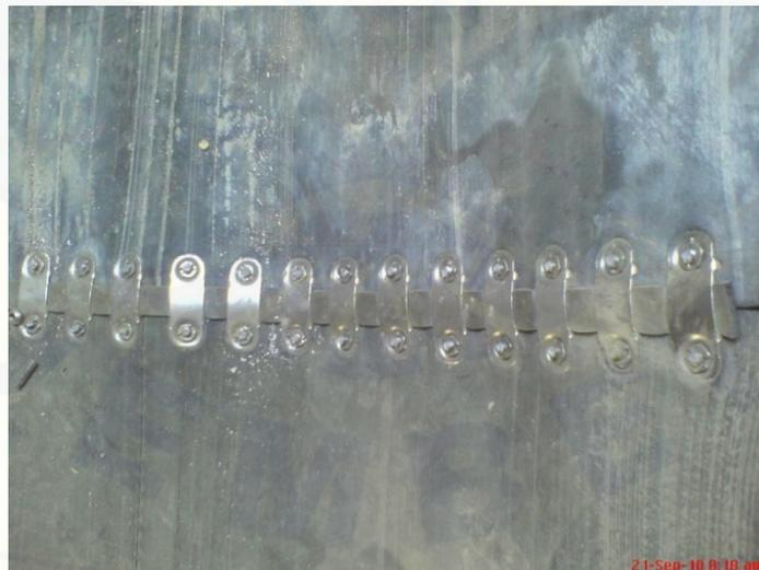
Gambar 2.8 Penyambungan *Mechanical System* (Sumber: *Summa Learning Center*)
