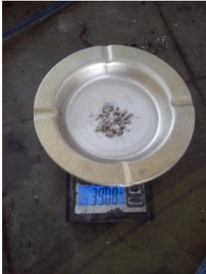
Gambar C.11 Hasil pengujian kadar abu tertinggi briket P 100
