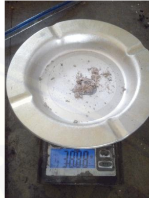
Gambar C.12 Hasil pengujian kadar abu terendah briket P 200
