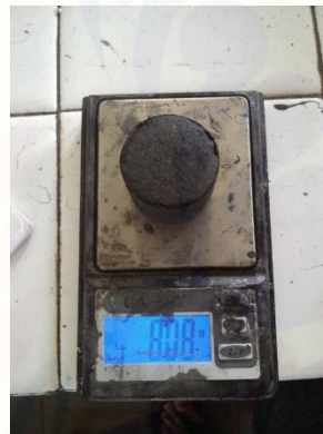
Gambar C.14 Hasil pengujian kadar air terendah P 200
