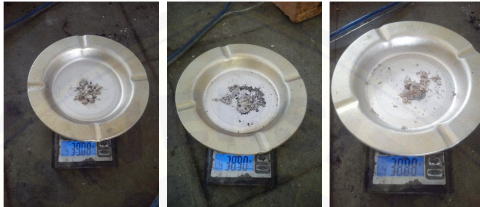
Gambar 4.5 Hasil pengujian kadar abu briket A (a), briket B (b), dan briket C (c)
