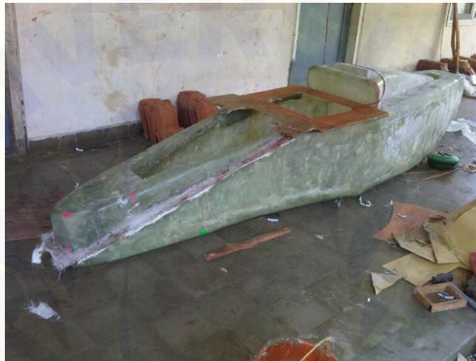
Gambar 2.11 Bodi Mobil Irit (Mobil Irit Universitas Jember)
